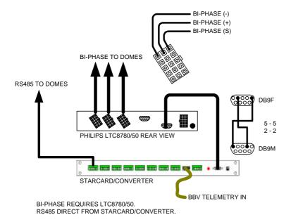
Set the dome address using the rotary switches to match the number of the camera input of the TX1500. Ensure that any dome at the end of a daisy chained RS485 run has the RS485 terminated and the intermediate domes have the RS485 de-terminated. If the dome only supports FastAddress<sup>TM</sup>, a Philips controller must be used to set the dome address before installation. The starcard/converter will not set the FastAddress<sup>TM</sup>.
