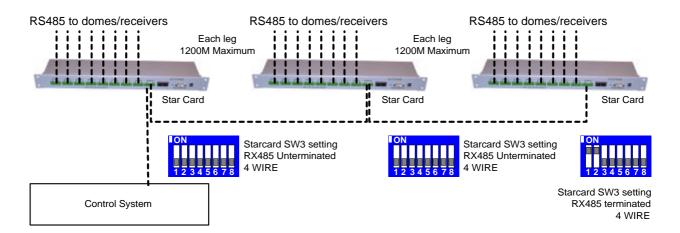
On single direction RS485, multiple StarCards can be daisy chained to provide multiple outputs.
